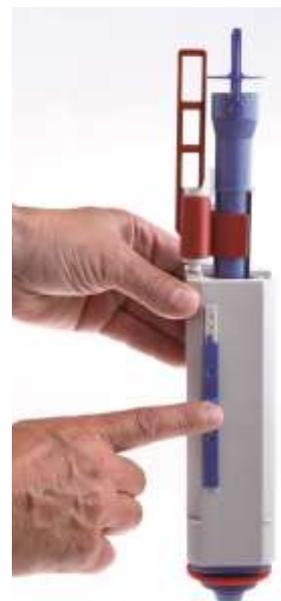
The red pull rod operates the reduced flush, the blue rod the full flush. The valve can be set to a full flush of 4.5, 6 or 9 litres at any time using the slider on the side, while the reduced flush of 3 litres always remains constant.
