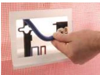
Undo the hose connected to the inlet valve and remove grey outlet valve hold down device.
